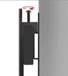
Arms feature levelling screws to adjust the screen height
