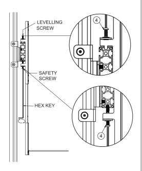
Important: 13mm or higher spacers are required for offsetting the screen when this shelf bracket is used together with the BT8390-VESA200F, BT8390-VESA200T, BT8390-VESA400F and BT8390-VESA400T.
