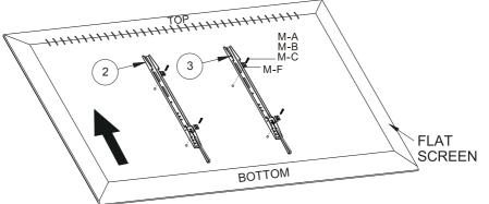
Lay screen flat on the floor (use cloth to prevent scratches to screen). Align interface arms to fixing holes on rear of screen, choose the appropriate size and quantity screws (with multi-washer) according to the mounting holes on screen.
