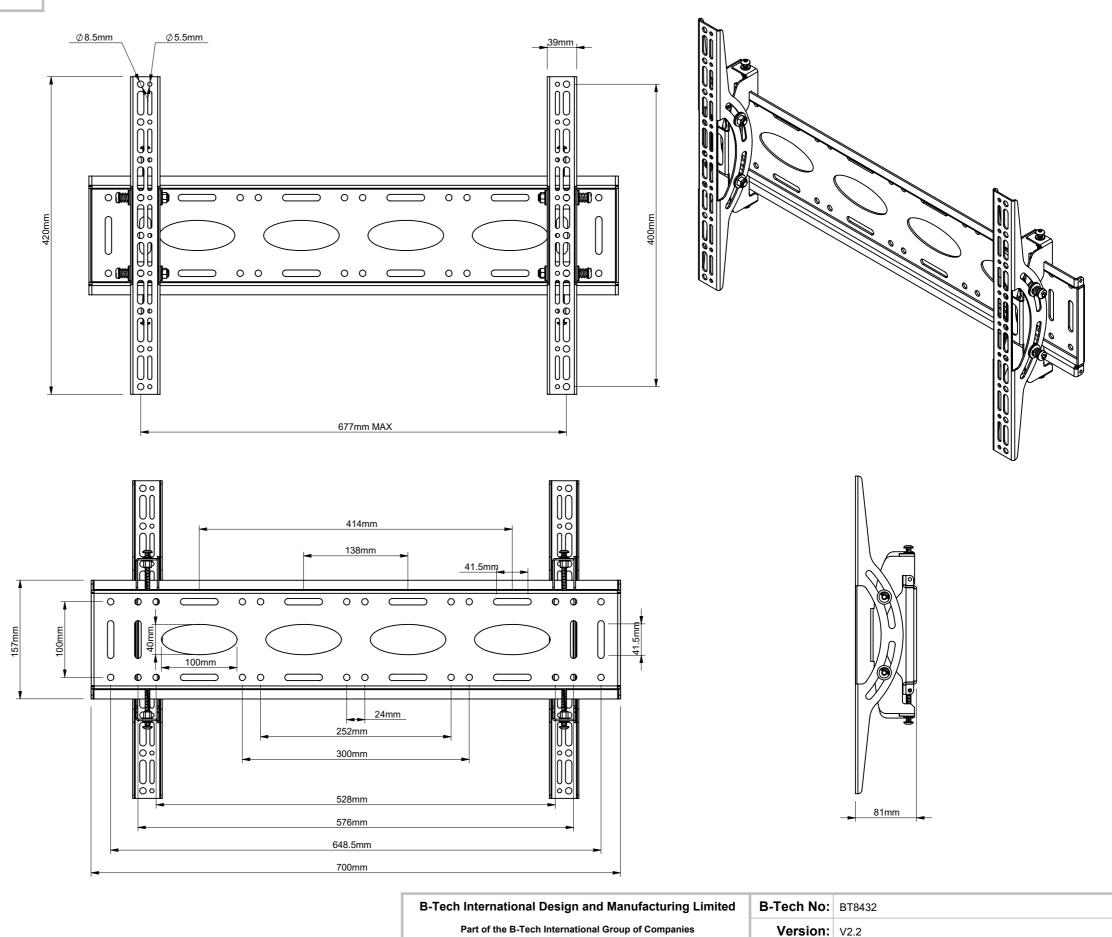
UNLESS OTHERWISE SPECIFIED DIMENSIONS ARE IN MILLIMETERS
