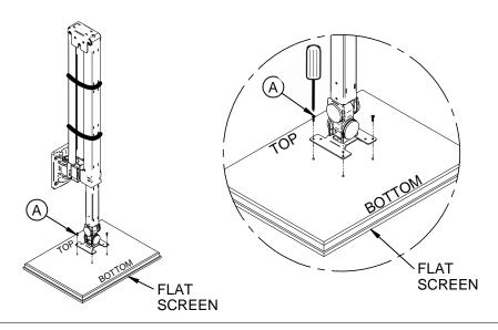
4 Remove the banding and release the safety lock so the articulating arm is free to move.
