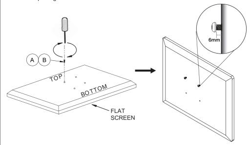
ii. Hook screen onto interface plate (Part 4), add bottom two screws and then tighten all screws.
